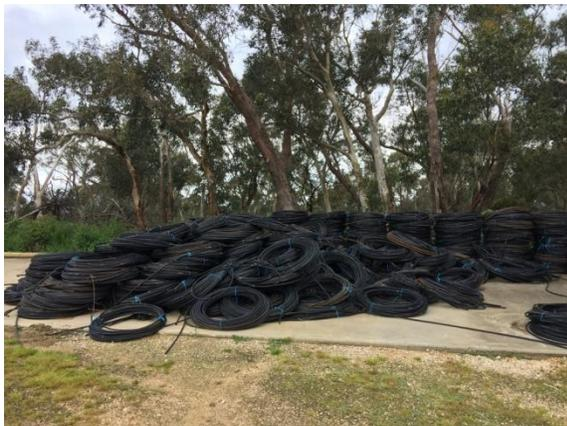
**Not so well recoiled** end-of-life polypipe in large open coils. Due to a less dense load, transport costs increase on a per tonne basis and the rebate returned to Grower, if any, is very small. Ongoing pick-up service viability is affected.
